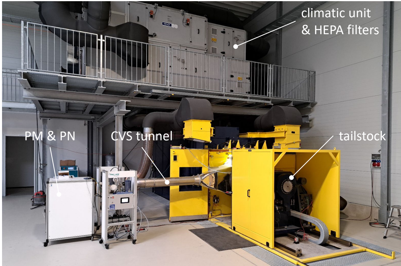
overview of dyno setup (showing emissions upgrade)
