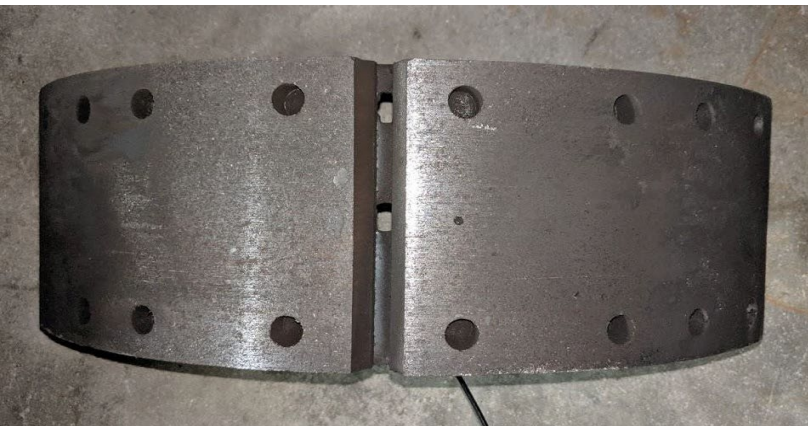
Thermocouples in primary brake shoes of all wheels per FMVSS 121
