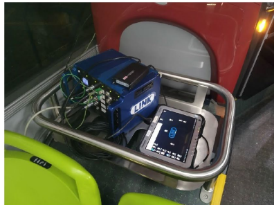
Figure 2: LINK VMAX Data Acquisition System
