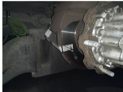
Figure 6: Thermocouple installed at the brake
