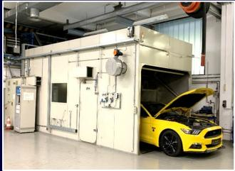
Testing of cars, light commercial vehicles and motorbikes under different climatic conditions
