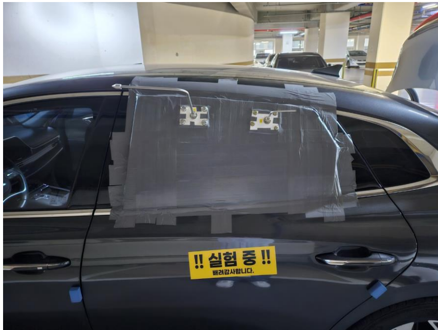
The outdoor air inlet and vent line
