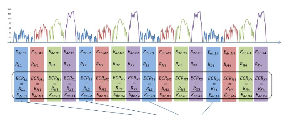
$E_{dc.mN}$  Total discharge energy [kWh]  $R_{mN}$  Driven distance [km]  $ECR_{mN}$  Energy Consumption Ratio [km/kWh] USA Usable Battery Energy from begging to end of test criteria [kWh]
