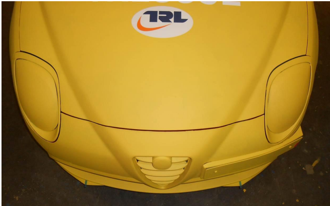
Figure 3-4: Alfa Romeo MiTo after having been measured for this task, showing the location of the 60° bumper corners as marked with green tabs.
