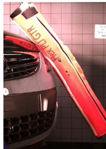
Figure 3-9: Motion of Flex-PLI during tests to end of bumper beam of Vauxhall Corsa: longitudinal test (Test 2) on left, normal test (test 3) on right
