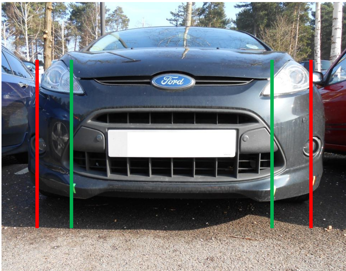
Figure 3-5: Ford Fiesta with the bumper corners shown as determined with a 60° plane (green) and a 45° plane (red).
