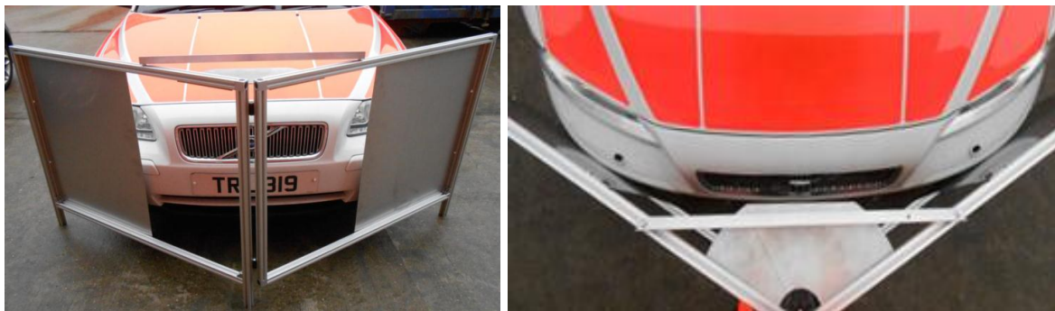
Figure 3-3: Collapsible frame being used to measure the length of the testable area between bumper corners on a Volvo V70.
