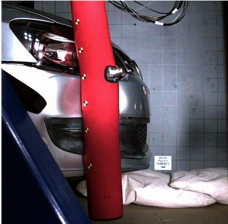
Figure 3-7: Volkswagen Polo during testing of the bumper corner defined by the 45° plane.
