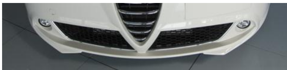
Figure 2-3: Example of a popular supermini car (Alfa Romeo MiTo) displaying additional front bumper designs that affect the definition of the bumper corners.
