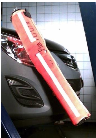
Figure 3-9: Motion of Flex-PLI during tests to end of bumper beam of Vauxhall Corsa: longitudinal test (Test 2) on left, normal test (test 3) on right
