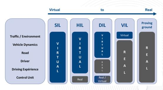
2. Carrying out "massive" simulations making it possible to cover a large number of driving situations and in particular the most dangerous or difficult to carry out in a real environment.
