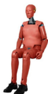
Procedures for Assembly, Disassembly, and Inspection (PADI) of the BioRID II Rear Impact Crash Test Dummy
