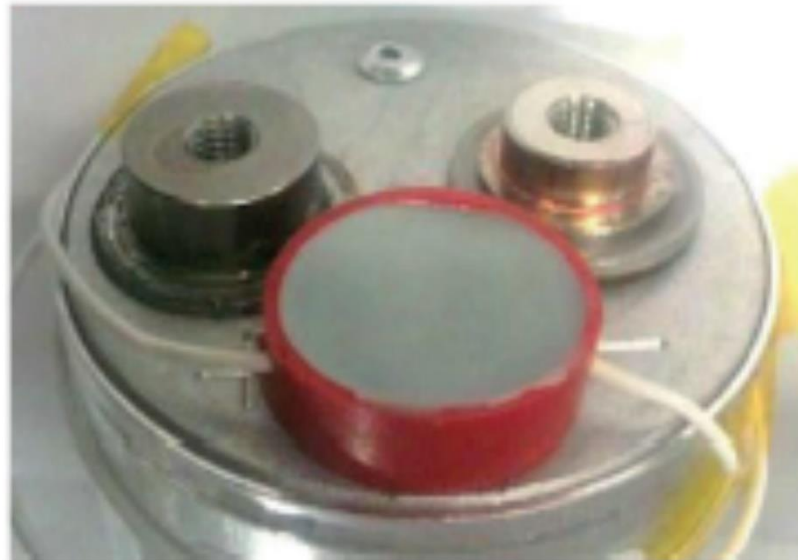
Figure 8 Example of cell before filling with electrolyte.
