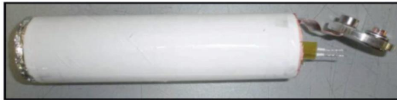
Figure 6 Example of jelly roll equipped with heater
