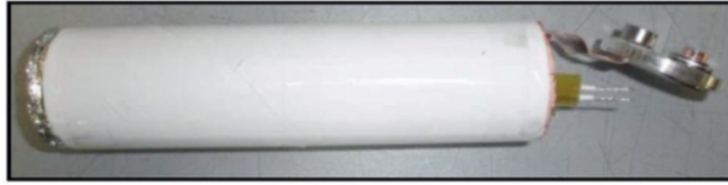
Figure 6 Example of jelly roll equipped with heater
