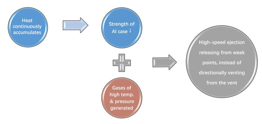
✓ Proposal: Prefer other methods to trigger Ni-rich NCM and HV NCM with a risk of Al case melting or any other performance degradation under external heat
