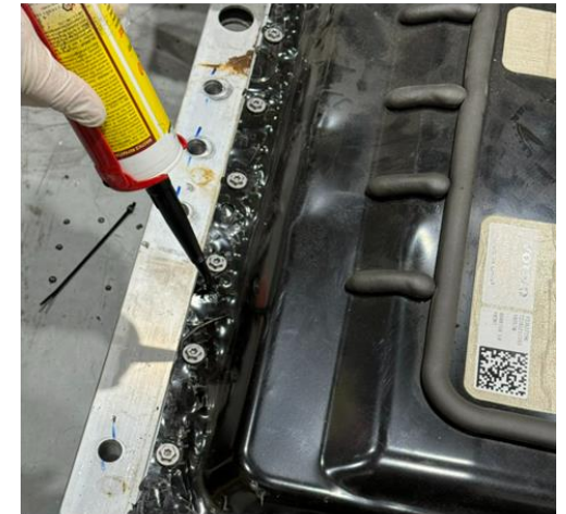
< Epoxy silicone application before/after attaching pack cover >
