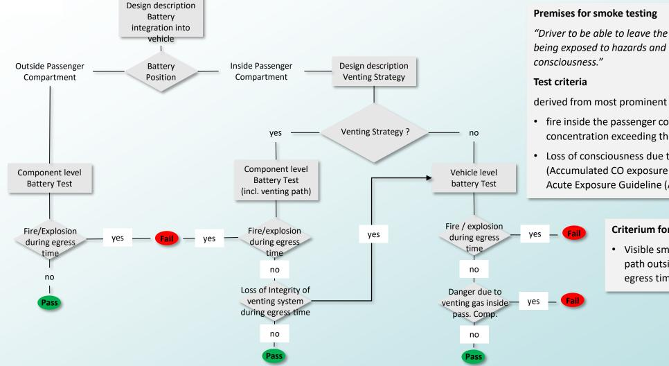
"Driver to be able to leave the vehicle during egress time without being exposed to hazards and without impediment of
