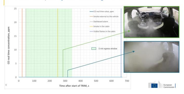
Detection of carbon monoxide (CO) within the cabin occurred after 650 seconds.
