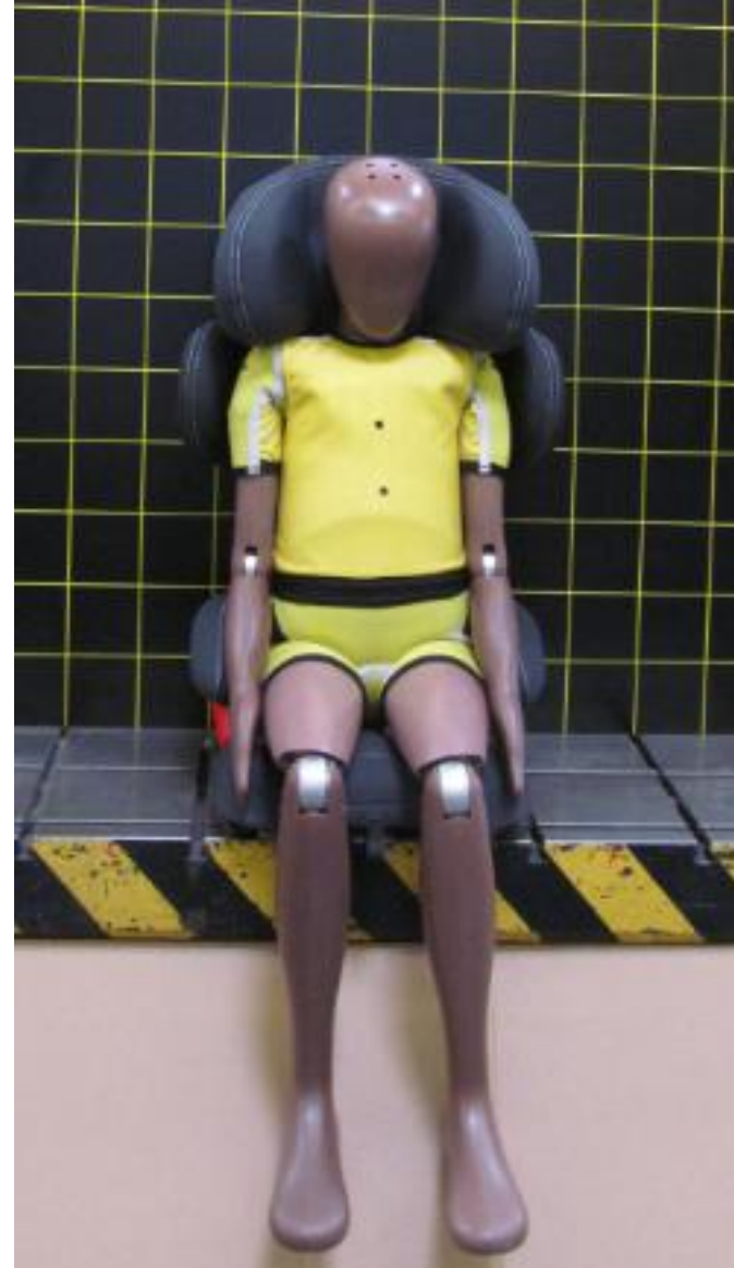
Q10 position is 1 notch below maximum extended
