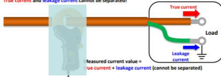
Figure 2. When Measuring the Current of a Wire with a Shielded Wire as is
