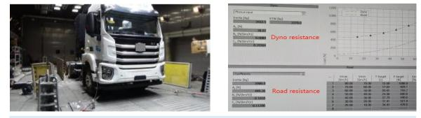
Coastdown test is simulated on chassis dynamometer to determine the set resistance coefficient A, B, C
