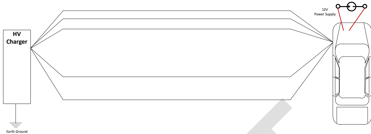
Figure 7 - 12V Power Supply Connection.
