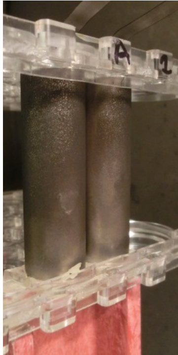
Figure 9 - Cylindrical cell coupon (2 cells) after exposure to smoke from smoldering electrical wiring.
