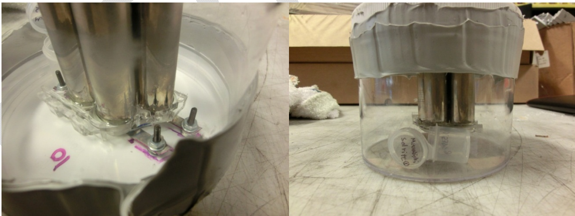
Figure 15 - An electrolyte exposure chamber containing 4 18650 cells after 20 days of exposure. Cloudiness can be seen on the cell walls due to the electrolyte vapor.
