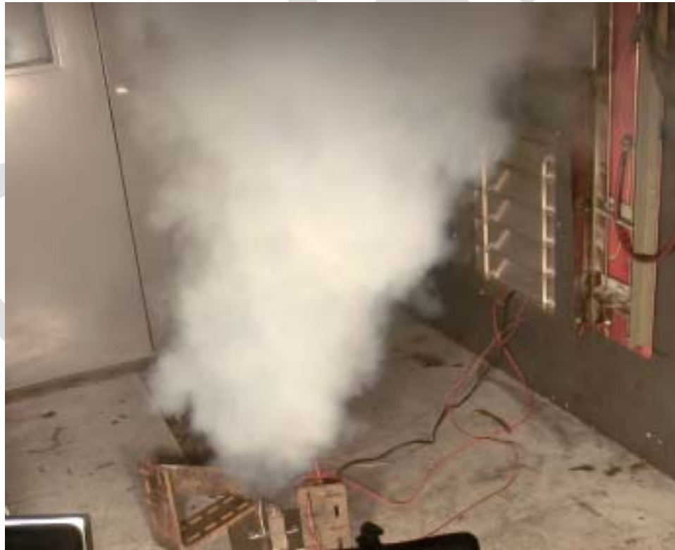
Figure 62 - Prismatic cell during thermal runaway; Large Film Heater Trial #1.
