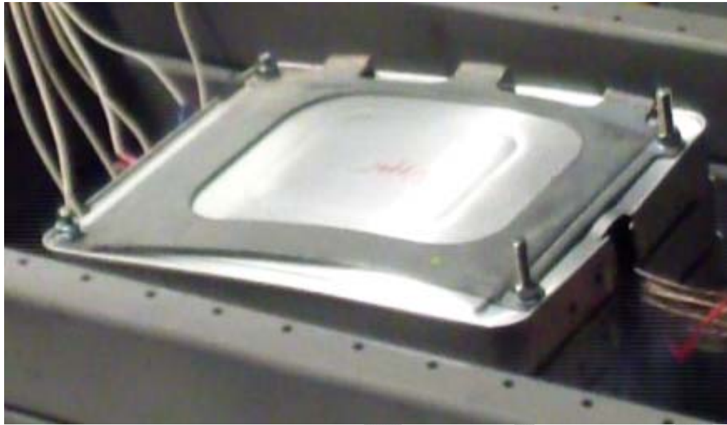
Figure 92 - Deformation of pouch cell Three Module stack.
