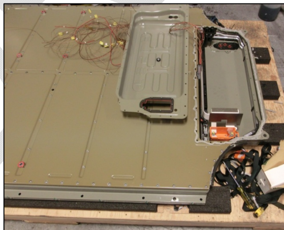
Figure 99 - The cylindrical battery pack, with sealant applied to seal the flat main cover to the front cover.
