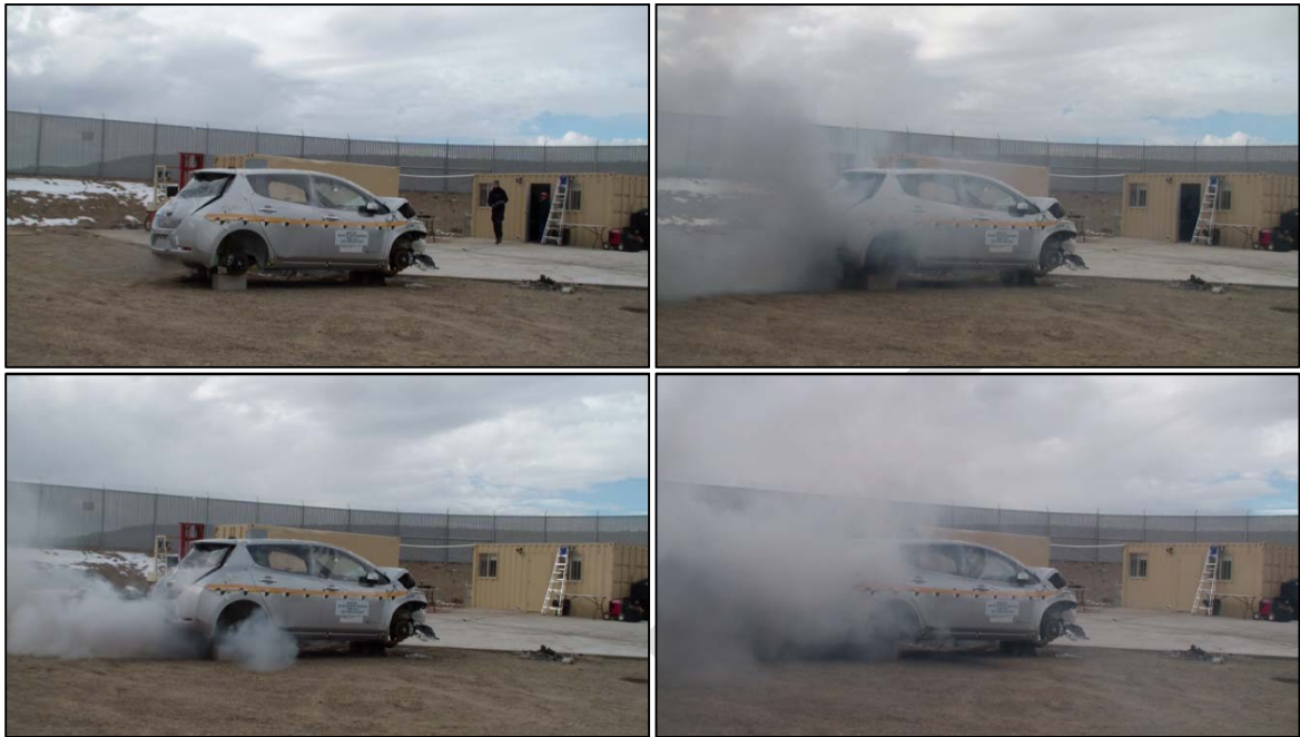
Figure 124 - Top left: 7:07, beginning of first runaway. Top right: 8:16, fourth cell runaway in the first module. Bottom left: 14:47, second module begins after lull. Bottom right: 22:10, several modules into event, ignition coming soon. Between runaways, the smoke cleared and resembled the top left image.
