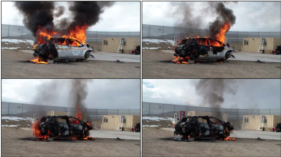
Figure 126 - Top left: 31:56, tallest flames. Top right: 36:04, vehicle fire concentrated in front. Bottom left: 46:03, event subsiding. Bottom right: 51:03, event nearing completion.
