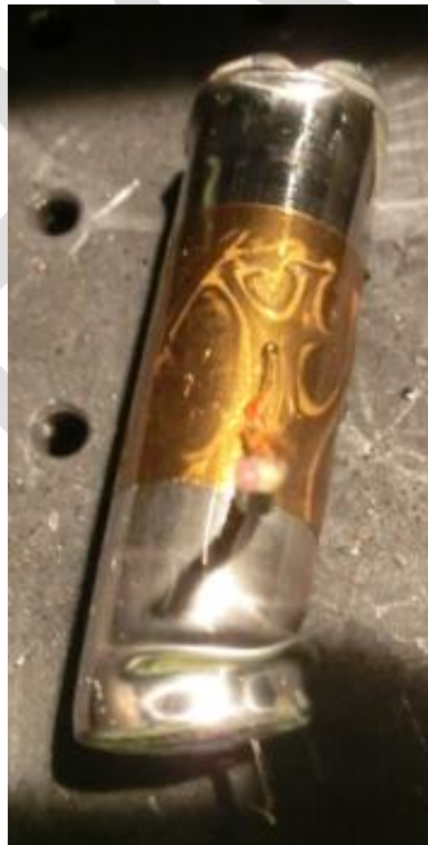
Figure 43 - Cylindrical cell after failed nail penetration trial.
