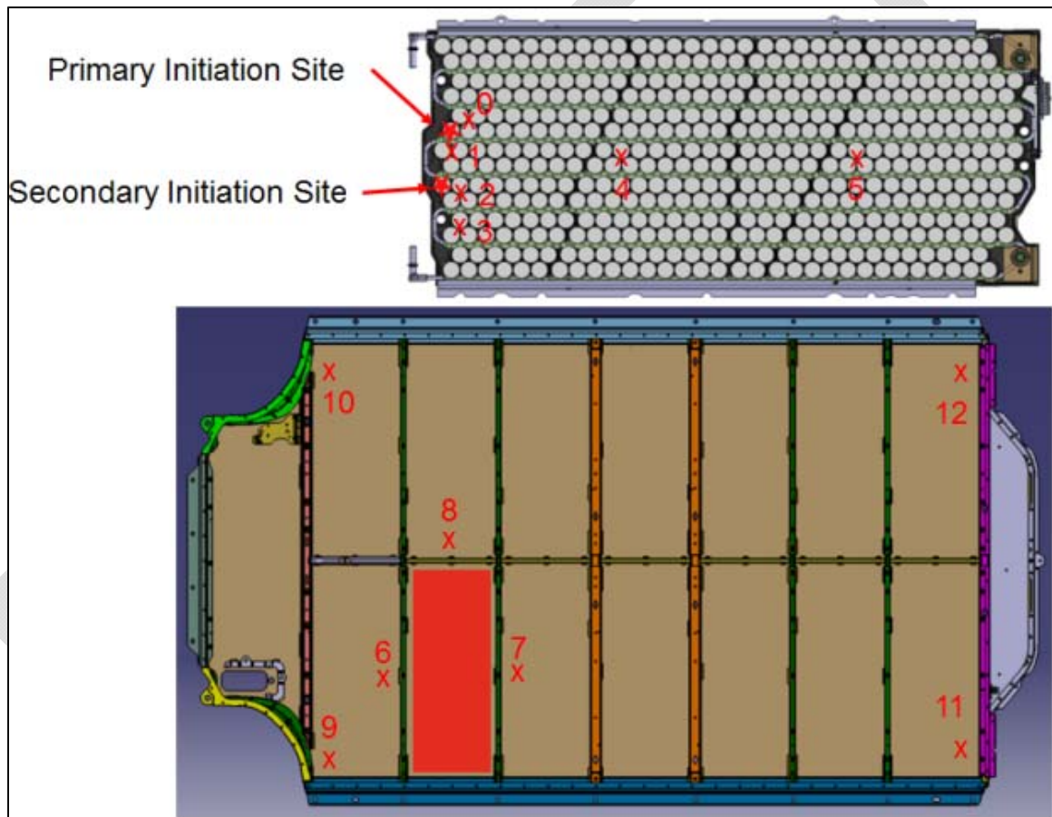
Figure 94 - Heater and thermocouple locations for the cylindrical battery pack.
