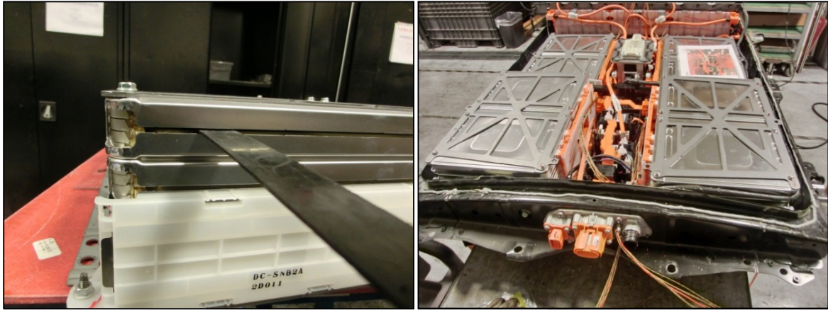
Figure 120 - Left: plastic strip used between the center two cells in a module to install a thermocouple. Right: all thermocouples routed through the pack, exiting through grommets, and the pack with a bead of sealant applied around the perimeter.
