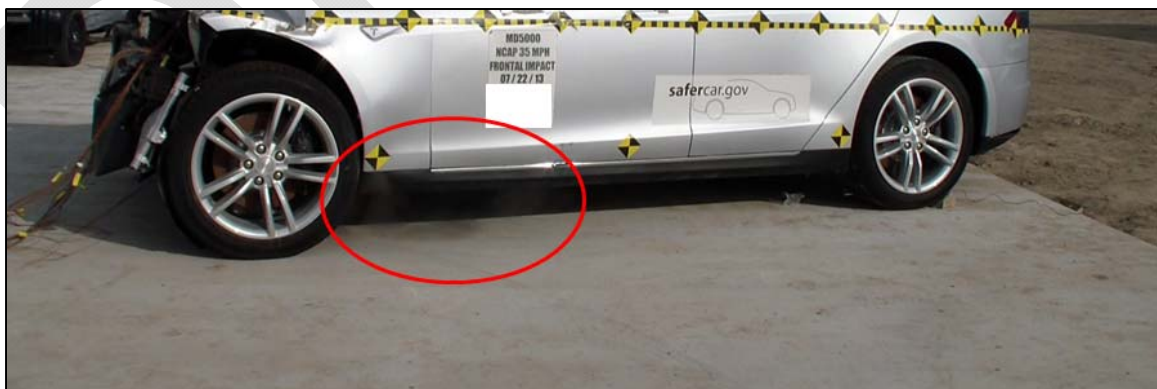
Figure 103 - Smoke escaping the battery pack as a result of thermal runaway of the initiating cell.
