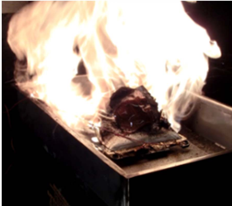
Figure 72 - Ignition of thermal runaway gases from pouch cell.
