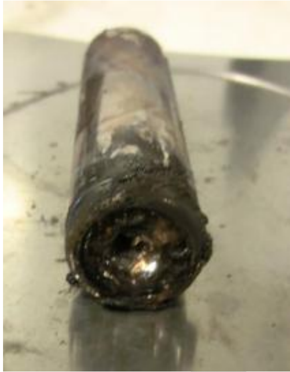
Figure 42 - Cylindrical cell after successful nail penetration trial.
