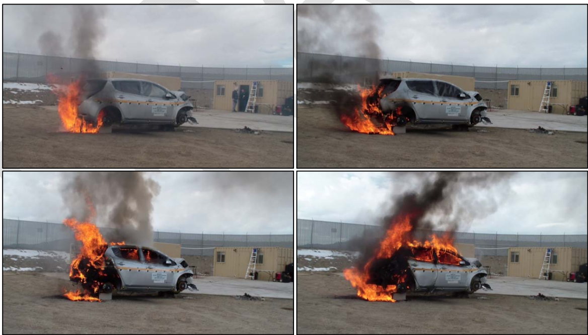
Figure 125 - Top left: 23:41, ignition has occurred. Top right: 26:44, rear flames continue. Bottom left: 28:22, flames inside cabin. Bottom right: 30:53, many internal flames.
