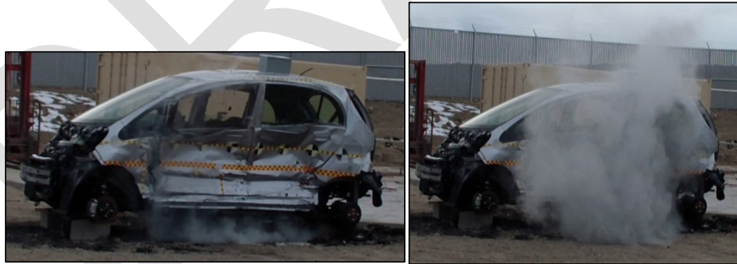
Figure 111 - Left: smoke starting during first runaway. Right: peak smoke emission during the first runaway.
