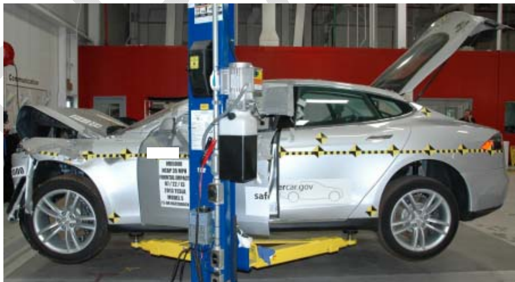
Figure 100 - The frontal crash Manufacturer A vehicle used for the demonstration of SCTRI testing.
