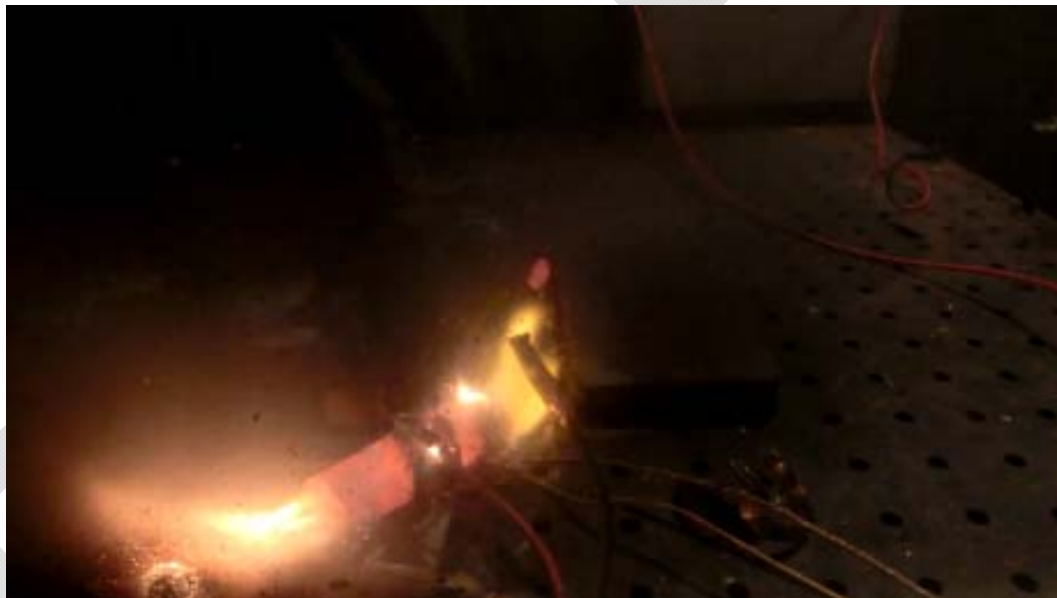
Figure 37 - Cylindrical Nichrome Wrap Heater cell immediately after runaway.
