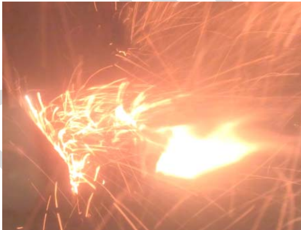
Figure 51 - Cylindrical cell undergoing thermal runaway, Off-the-Shelf Heater method.
