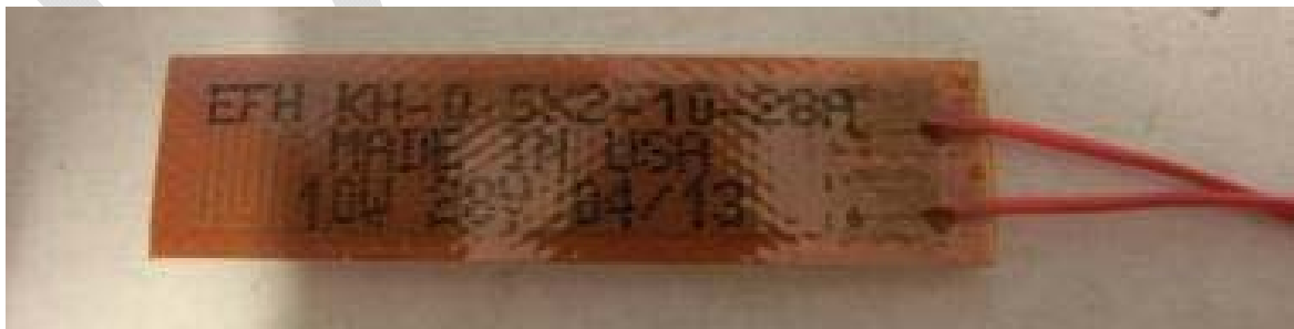
Figure 32 - Off-the-shelf film heater.
