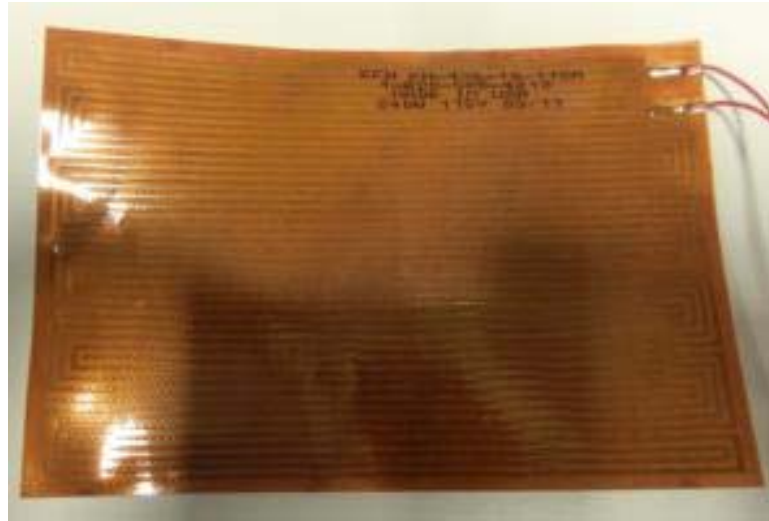
Figure 53 - Large off-the-shelf film heater.
