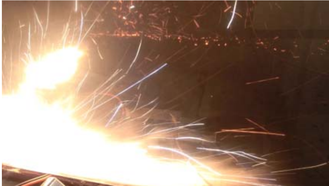
Figure 36 - Cylindrical cell undergoing thermal runaway; Nichrome Wrap Heater method.
