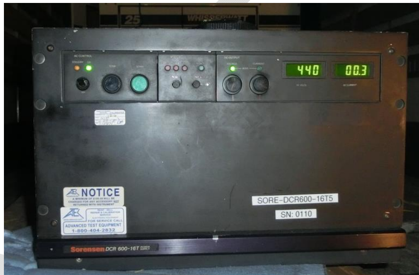
Figure 40 - The Sorensen DCR-600 DC power supply used for both over voltage and over current overcharge testing. It is rated for 600 V / 16 A (9.6kW).
