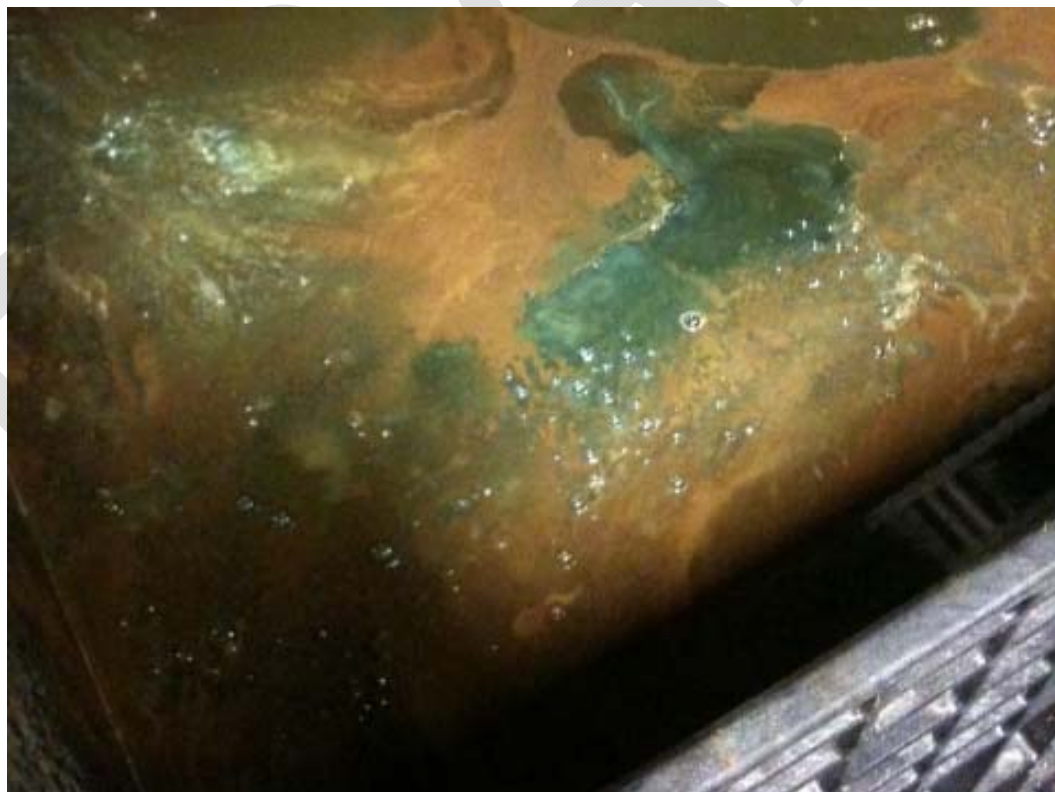
Figure 13 - Example of a salt bath with submerged modules: note bubbles of gas on surface produced by electrolysis.
