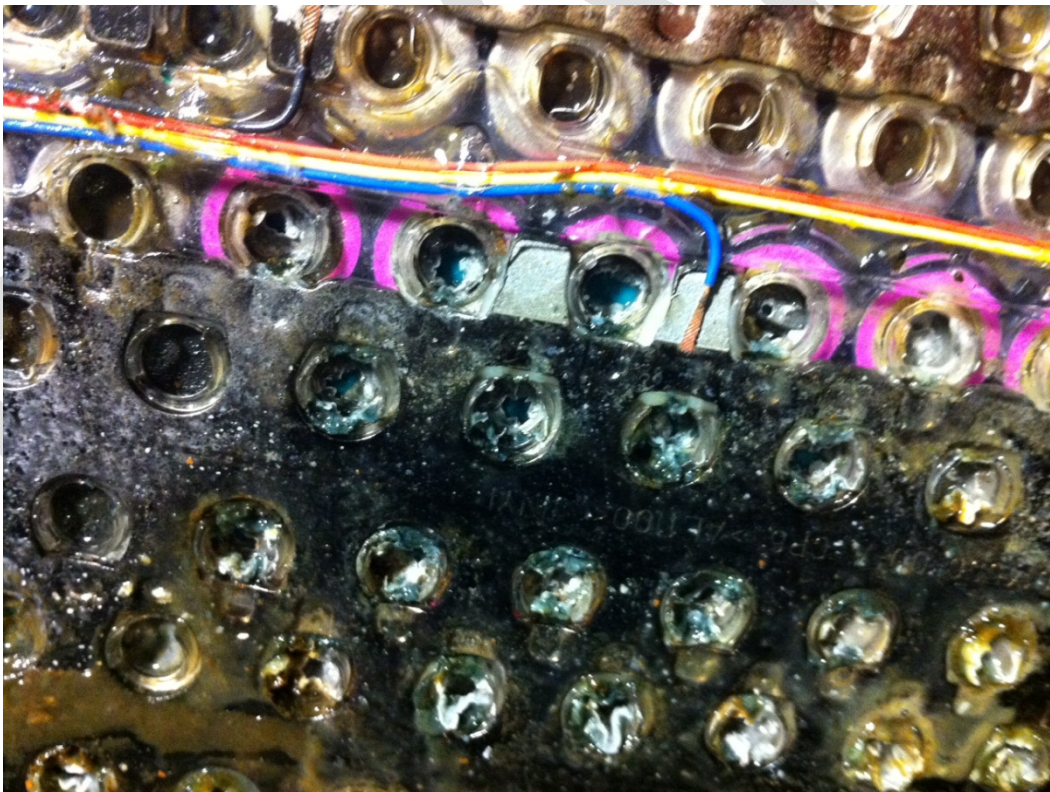
Figure 43 - Example of a Manufacturer A module after salt bath destructive discharge.
