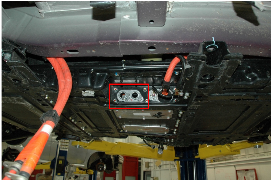
Figure 16 - Manufacturer B; high voltage cable pass through (red box) into RESS (high voltage cables have been disconnected and are hanging at left).
