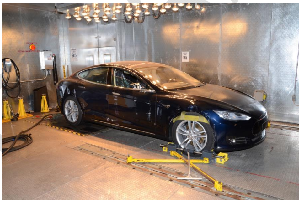
Figure 30 - The Test Vehicle as installed on the dynamometer. Solar load lights are used to provide illumination for the image, but were not used during testing. The Level 3 charge cable can be seen, coiled, at the left of the image.
