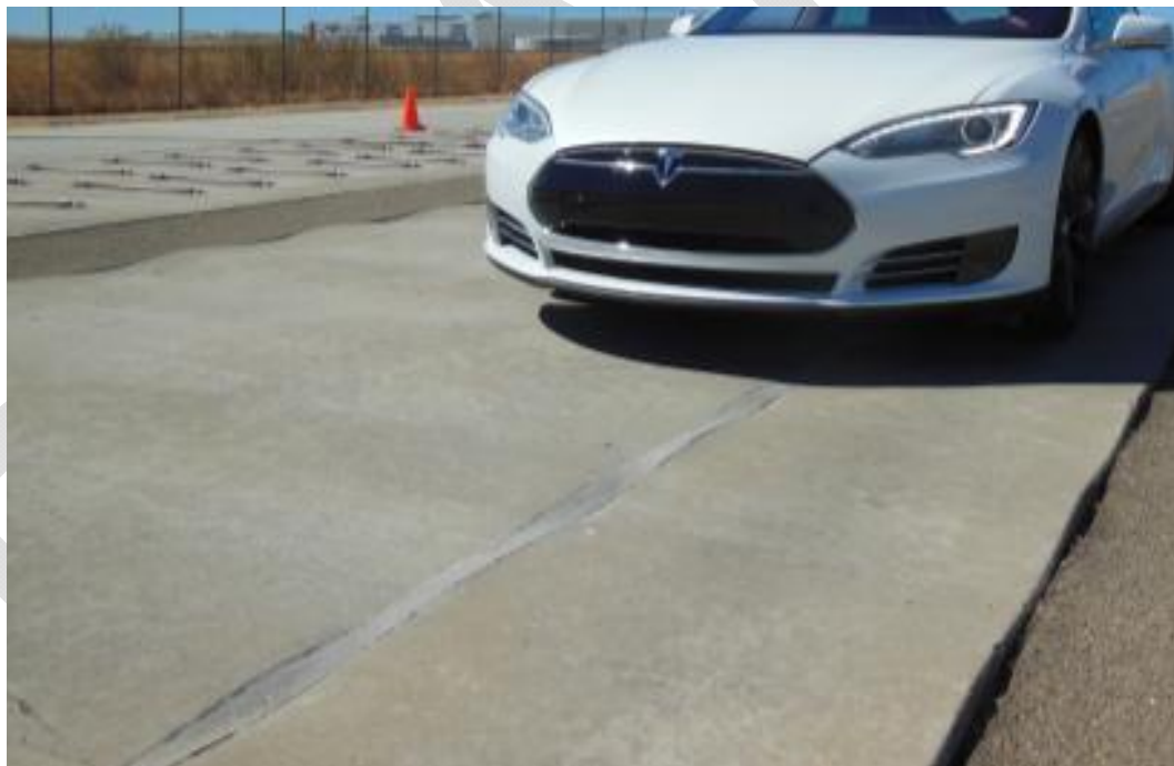
Figure 22 - Example of a vehicle on a wave / sinusoidal road (rough road element).
