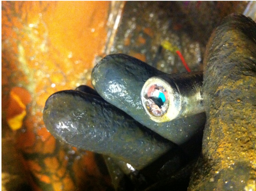
Figure 10 - Example of an 18650 cylindrical cell after salt bath destructive discharge: positive terminal has been removed by corrosion, exposing the cell interior.
