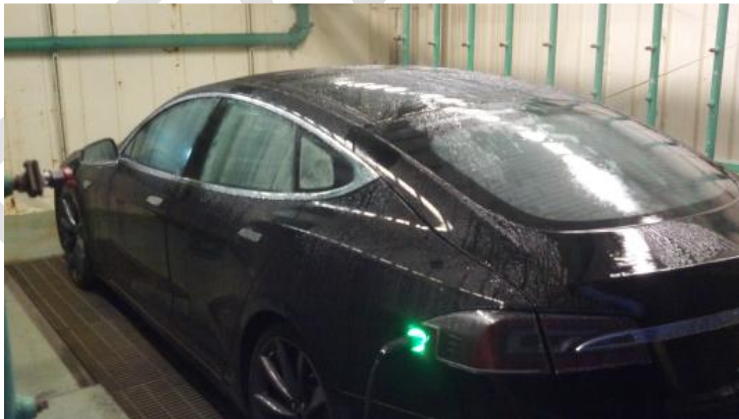
Figure 28 - Example of a vehicle subjected to drizzle chamber charging; drizzle is simulated by applying a total water flow rate of 12GPM from the top of the chamber only.
