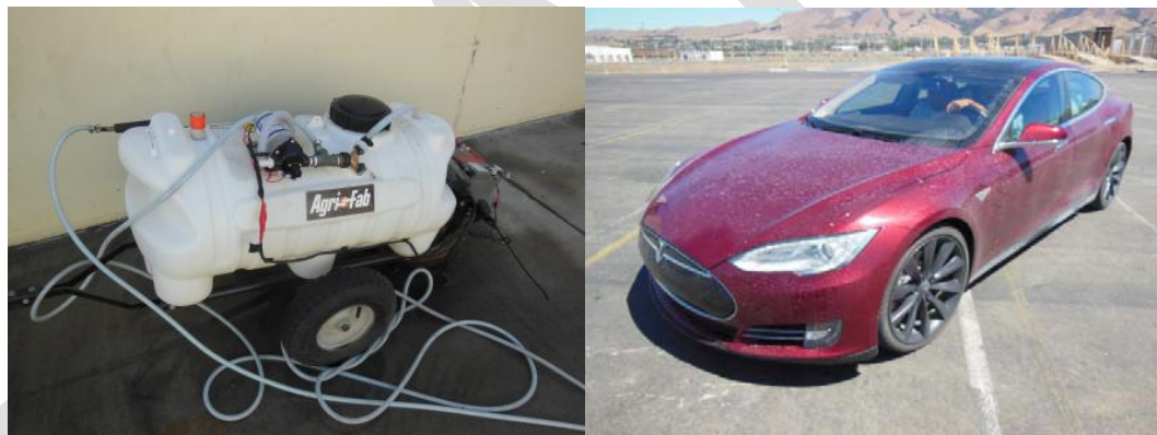
Figure 24 - Salt spray applicator and example of a vehicle after application of salt spray.
