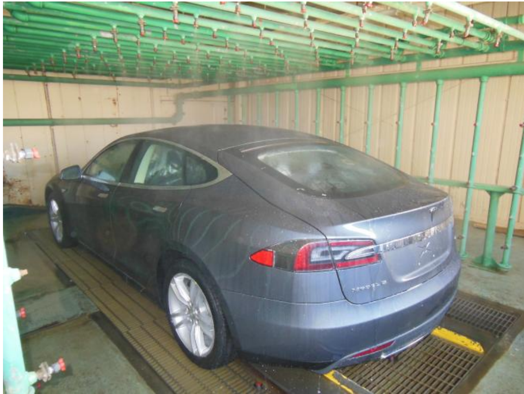
Figure 27 - Example of a vehicle installed in the booth used for rain and drizzle testing. Rain (monsoon) is simulated by applying a total water flow rate of 600 GPM divided into 150 GPM per side (top, left, right, bottom).
