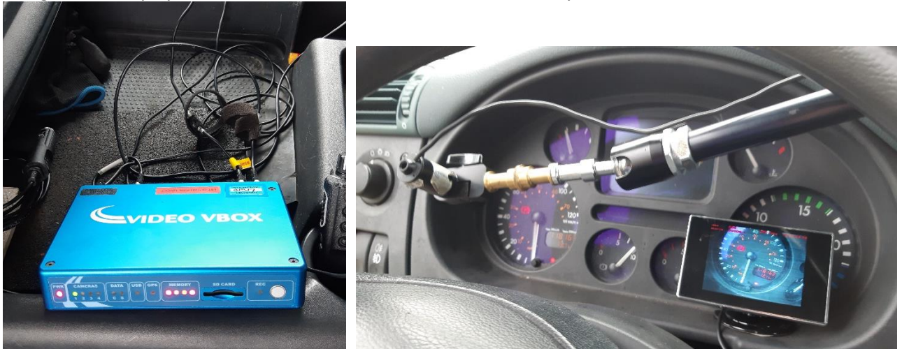
Figure 1: VIDEO VBOX and camera filming the odometer
