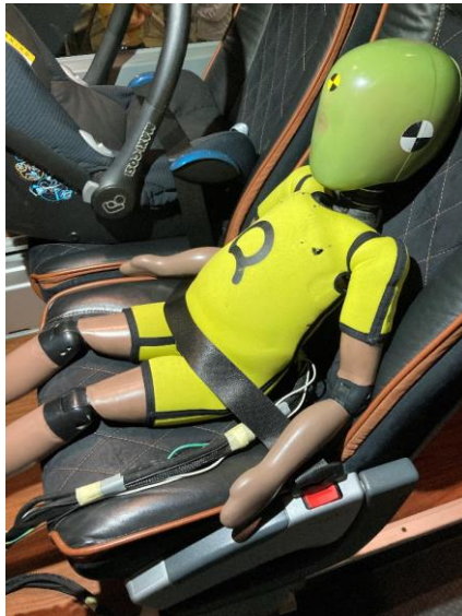
Q3 dummy on coach seat (no CRS)
