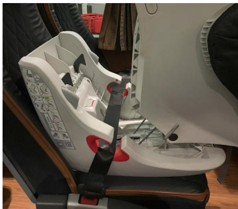
Forward-facing CRS (seating unit lifted to allow access to belt route)
