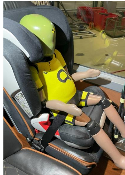
Q3 dummy on booster seat
