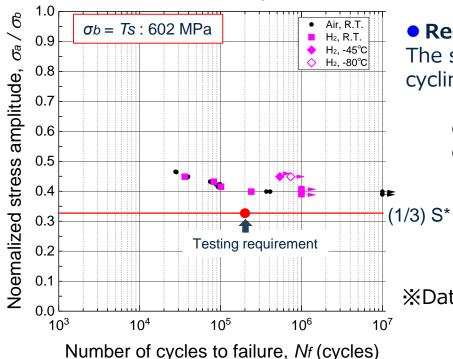
• Requirement for fatigue life test of Option 2
