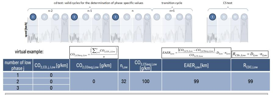
**R:** The  $CO_{2,CDavg,Low}$  will always be zero if there is no power-triggered engine start because the transition cycle is excluded. That means  $EAER_m$  equals  $R_{CDC.m}$ !
