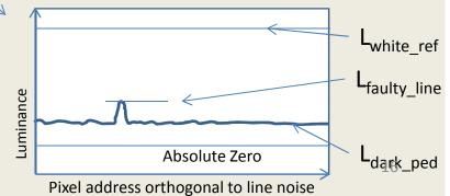
Artificially generated image to see the impression of what a vertical bright line would look like. Actual image on a working CMS may look difference due to further random noise and Dark pedestal level.
