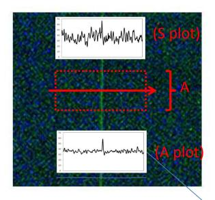
Fixed color noise of this type occurs mainly as result malfunctioning of the sensor reset, read out, vertical line amplification circuit.
