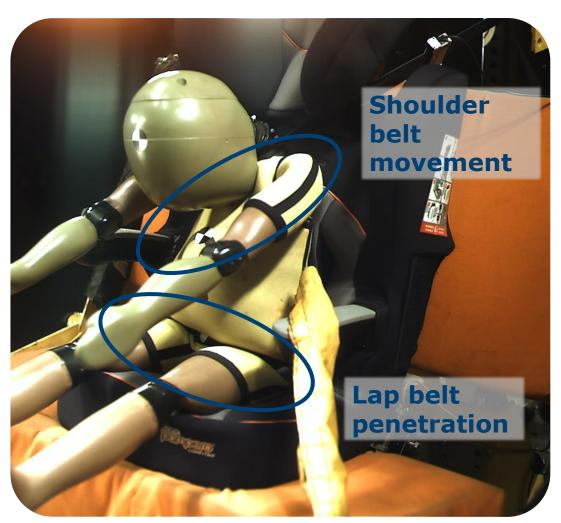
Diagonal belt loads dummy away from deflection sensor – limit belt movement or 2<sup>nd</sup> sensor needed?
