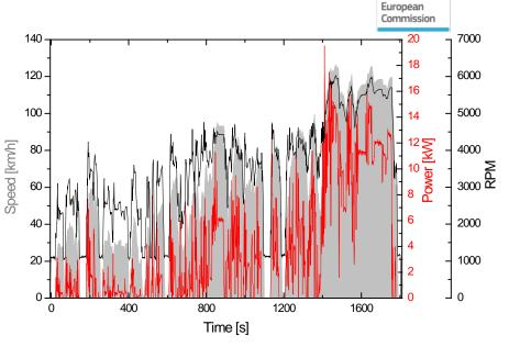
Vehicle 4 on different driving cycles: ECE-40, WMTC, Full Power
