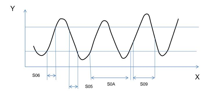
Example for where each data is monitored Judge the deterioration by monitoring the signal variation
