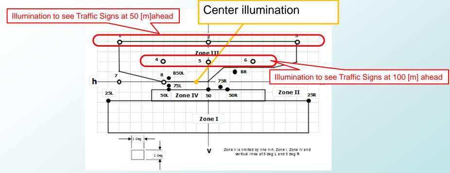
Requirement to avoid glare and keep minimum illumination to observe the Traffic Signs.
