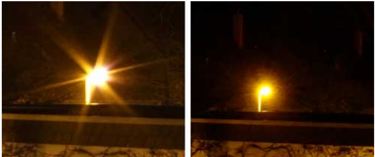
Figure 11: Flare effect (left small aperture, right large aperture)
