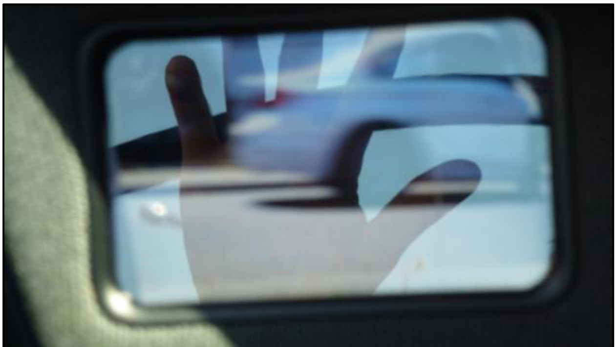
Figure 37: Reflections on the passenger side display.
