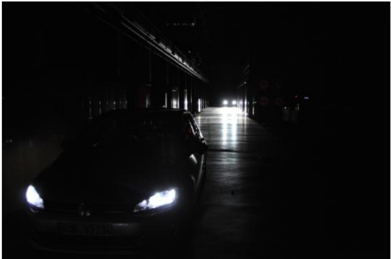
Figure 32: Test set-up: The following vehicle at a distance of 50 m with turned on dipped beam head lights.
