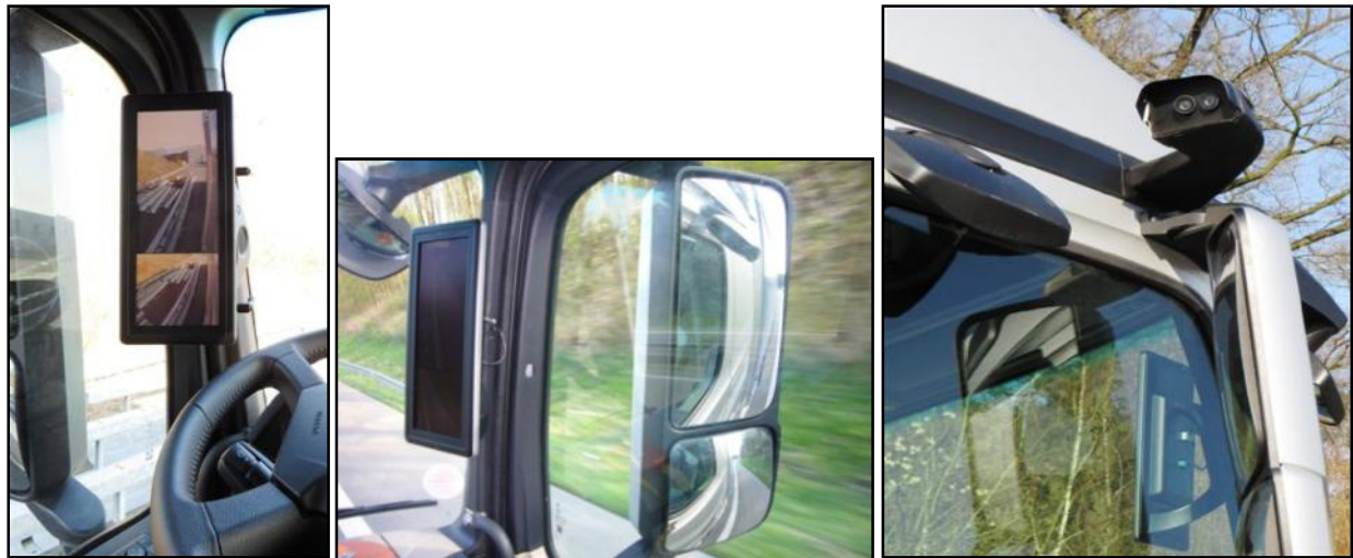
Figure 9: Exterior mirrors with cameras and monitor integration next to the A-pillar on a truck.
