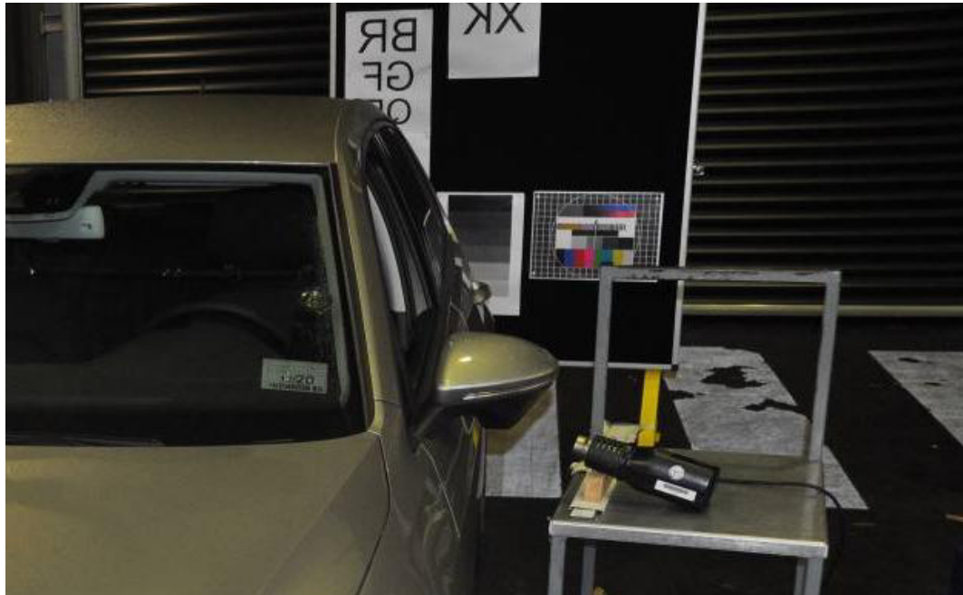
Figure 47: Test set-up for behaviour in extreme heat.
