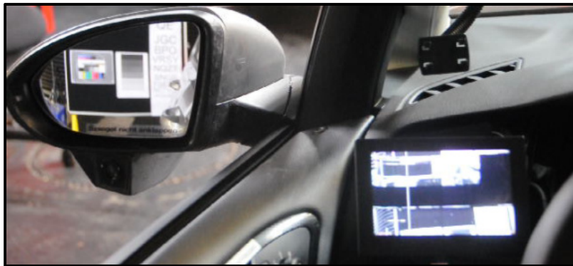
Figure 40: Error in image caused by electromagnetic radiation.
