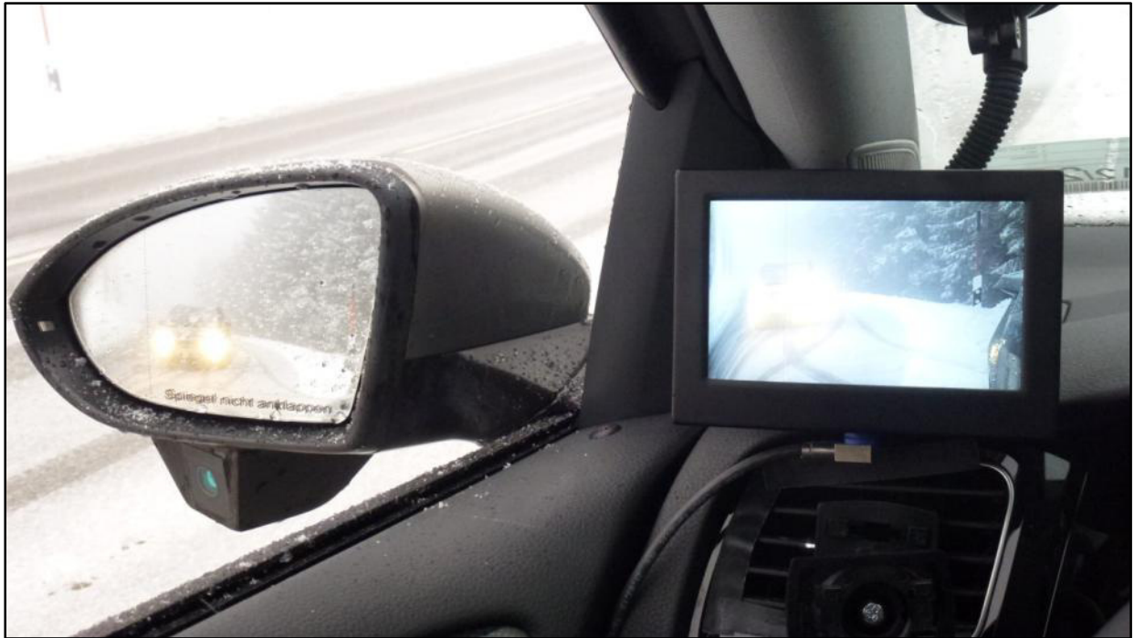
Figure 26: Comparison at snow fall and higher ambient luminance (close vehicle).
