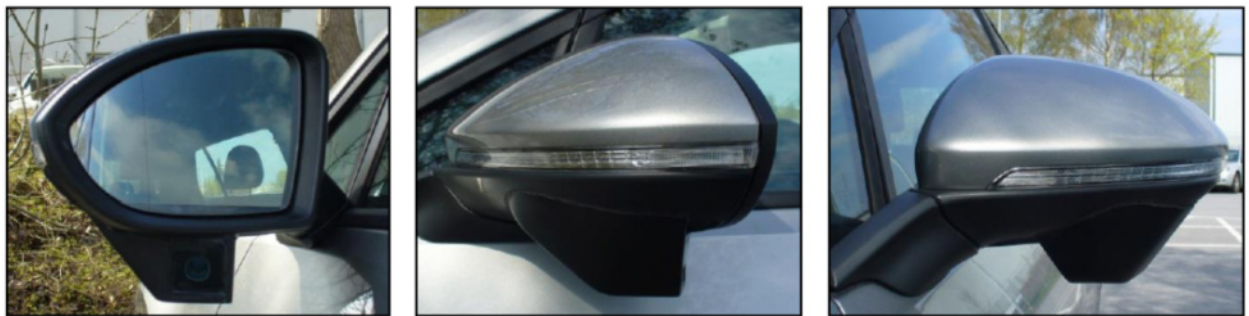
Figure 3: Left exterior mirror with camera mounted to the mirror housing.
