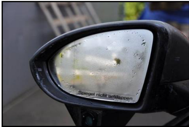
Figure 44: Camera and mirror fogged up.
