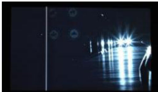
Figure 35: Monitor at a distance of 50 m and turned on high beam head lights.
