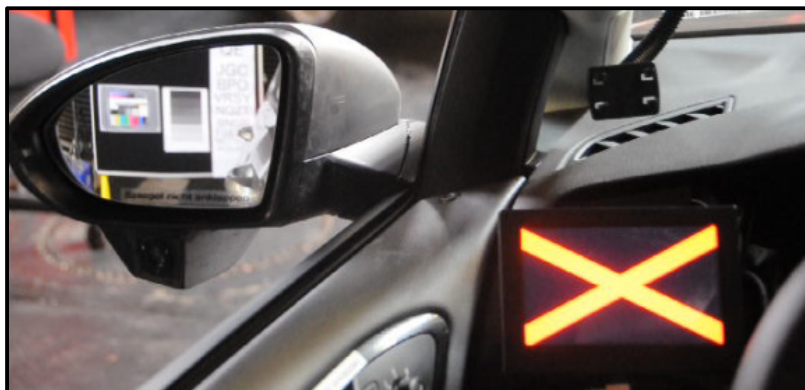
Figure 41: Loss of image caused by electromagnetic radiation.
