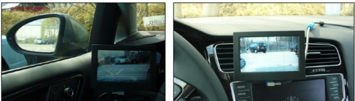
Figure 5: Integration of the monitors on the air vent grids (Position CMS 2).
