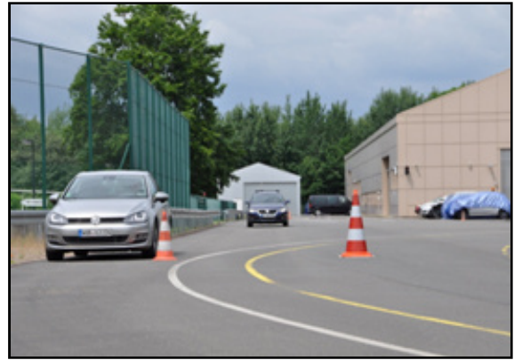
(b) Outside of the test vehicle: Object vehicle approaching from behind at a consistent speed.
