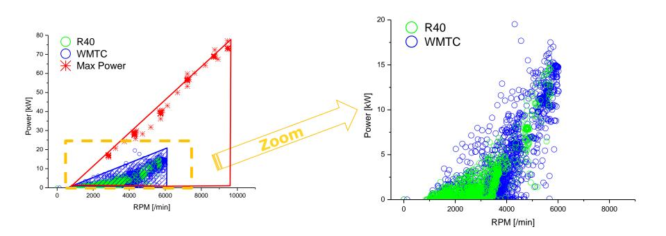
Larger area covered by WMTC  $\rightarrow$  maximized sampling in the part-load area
