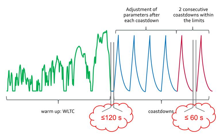
▶ Time between warm up and coastdown to start automation system, dynamometer, autopilot (...) shall be as short as possible.
