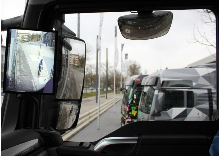
Figure 6: Comparison between the current mirror system and the developed CMS prototype on the passenger side of a commercial vehicle
