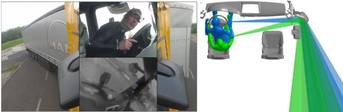
Figure 5: Expanded field of view by a bending forwards. Comparison of real and simulated behavior
