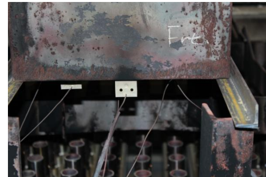
K-Type \varnothing 1.6mm / 25±5mm from the bottom of DUT
