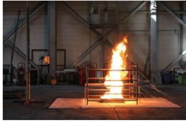
< Small pool-Burning with Mockup >
