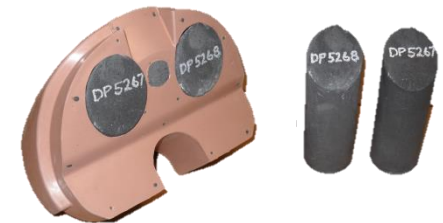
Q10 abdomen with foam cylinders for certification
