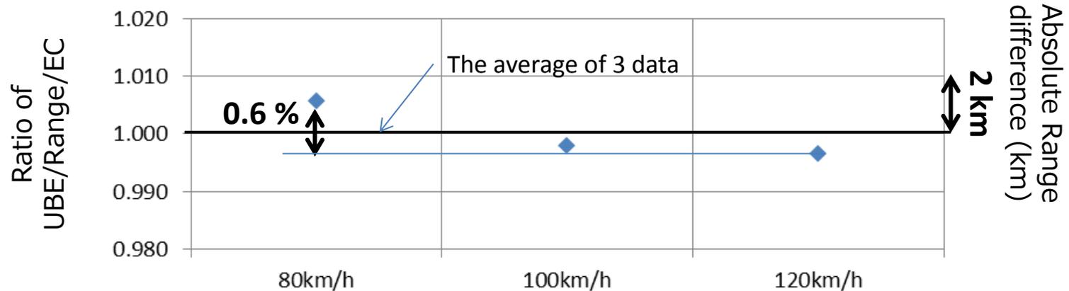
(reference) The battery temperature increases as CSC speed goes up. Thermal loss in cells is main contributor of UBE difference, but negligible within above speed range ( 80 ~ 120 km/h)
