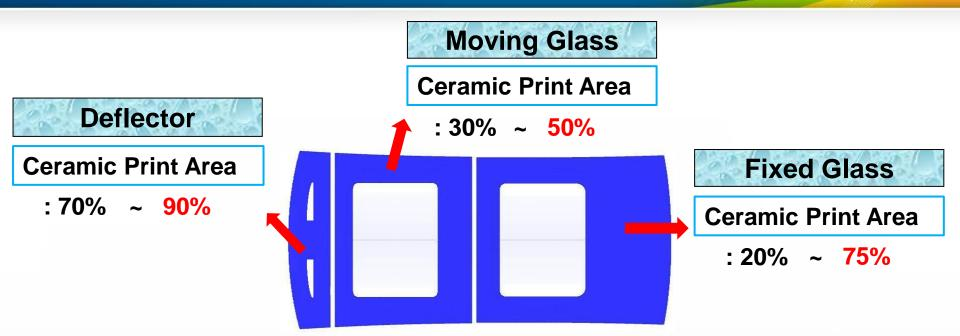
Ceramic printed toughened glass cannot be considered toughened glass as its strength is poorer than to original glass
