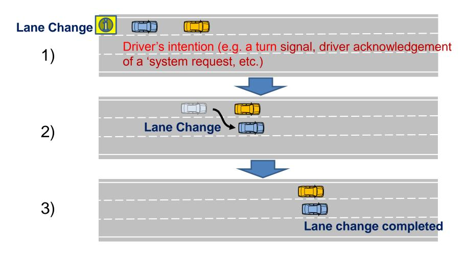
Note: When the driver operates LC switch, the vehicle moves to the target lane. After this movement, the operation of LC is finished.
