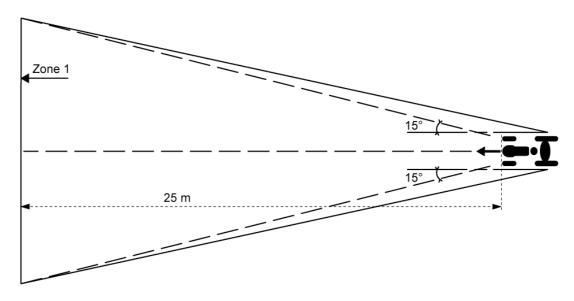
Figure 2 Visibility of a white lamp to the rear
