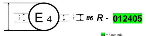
The above approval mark affixed to an agricultural or forestry vehicle shows that the vehicle type concerned has, with regard to the installation of lighting and light-signalling devices, been approved in the Netherlands (E 4) pursuant to Regulation No. 86. The approval number indicates that the approval was granted in accordance with the requirements of Regulation No. 86 in its original form as amended by the 01 series of amendments.
