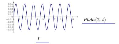
With the given values of depth and length of the individual pothole we look at the acceleration Ha() in the separation of the two vehicles. The length of the drawbar is as given above.
