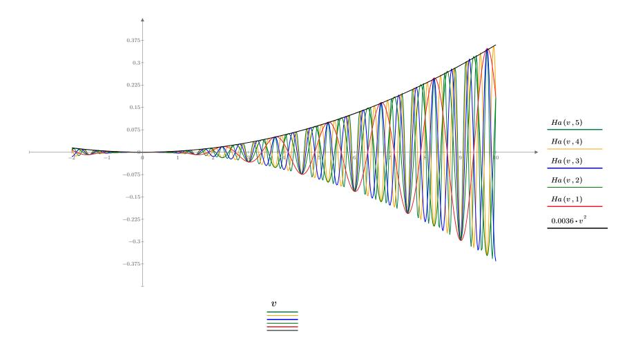
As the previous diagram may be hard to comprehand we also make a graph illustrating the variation of the acceleration as a function time at constant speed (2, 4, 6, 8 and 10 m/s). We than se the dependence of speed nicely illustrated. We note the frequency shift as the speed increases over the constant pothole series.
