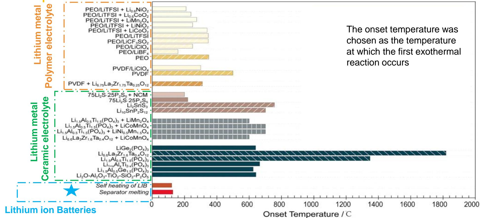
Cells with different chemistries have varying onset TR temperatures, some close to those of contemporary Li-ion technology
