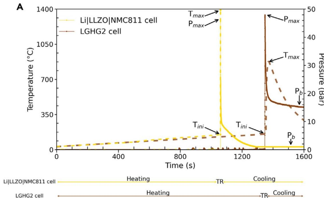
The cell is wrapped with a heating wire (9A power supply, 300V) to trigger TR
