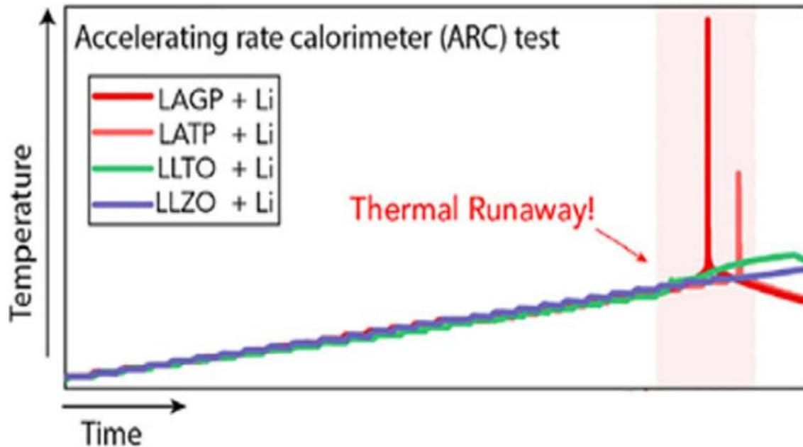
Thermal response of pouch cells with different SSEs
