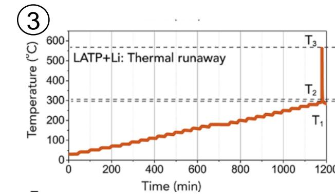
Triggering TR by heating the cell in the arc chamber
