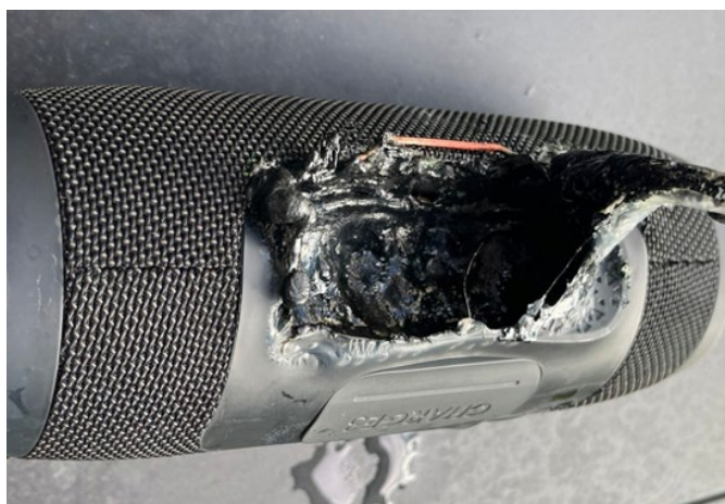
Figure 12 Bluetooth speaker where the embedded battery has caught fire (supplied)
