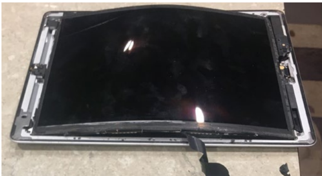
Figure 6 Tablet battery expansion when being charged by no brand charger is unable to manage its charge
