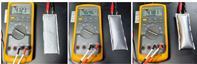
Figure 5 NMC lithium pouch cells responding to overcharging, where (left) is the normal voltage conditions and (middle and right) are beyond the safe operating conditions
