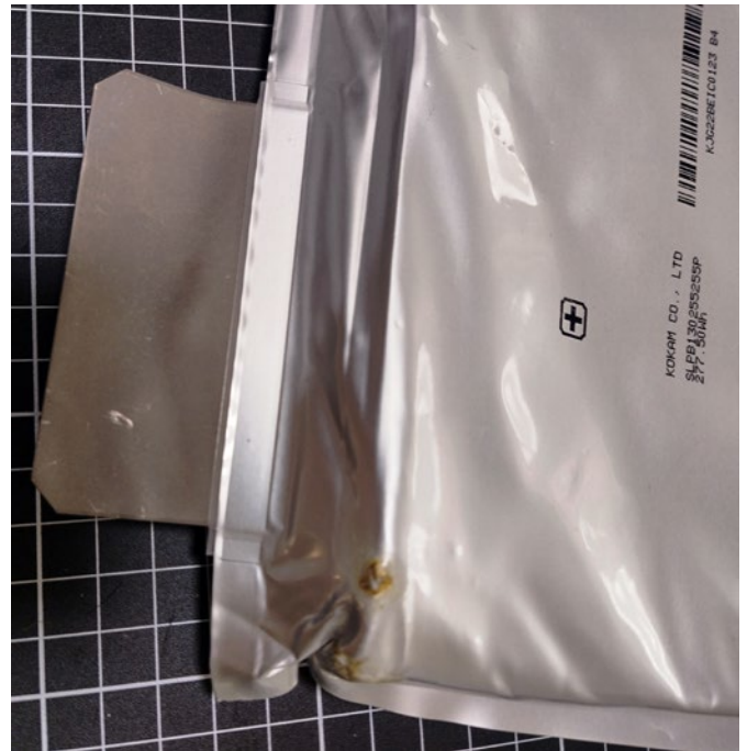
Figure 9 Damage to large high energy pouch cell due to impact at the corner
