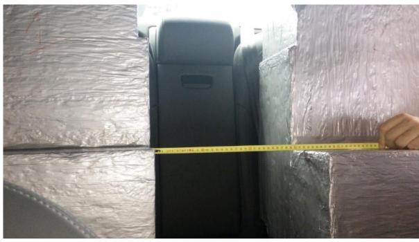
Audi A8 > 2 TF4 boxes of 520 mm. width fit; 3 boxes with a width of 440 mm. can fit, when only mounted with carbelt.
