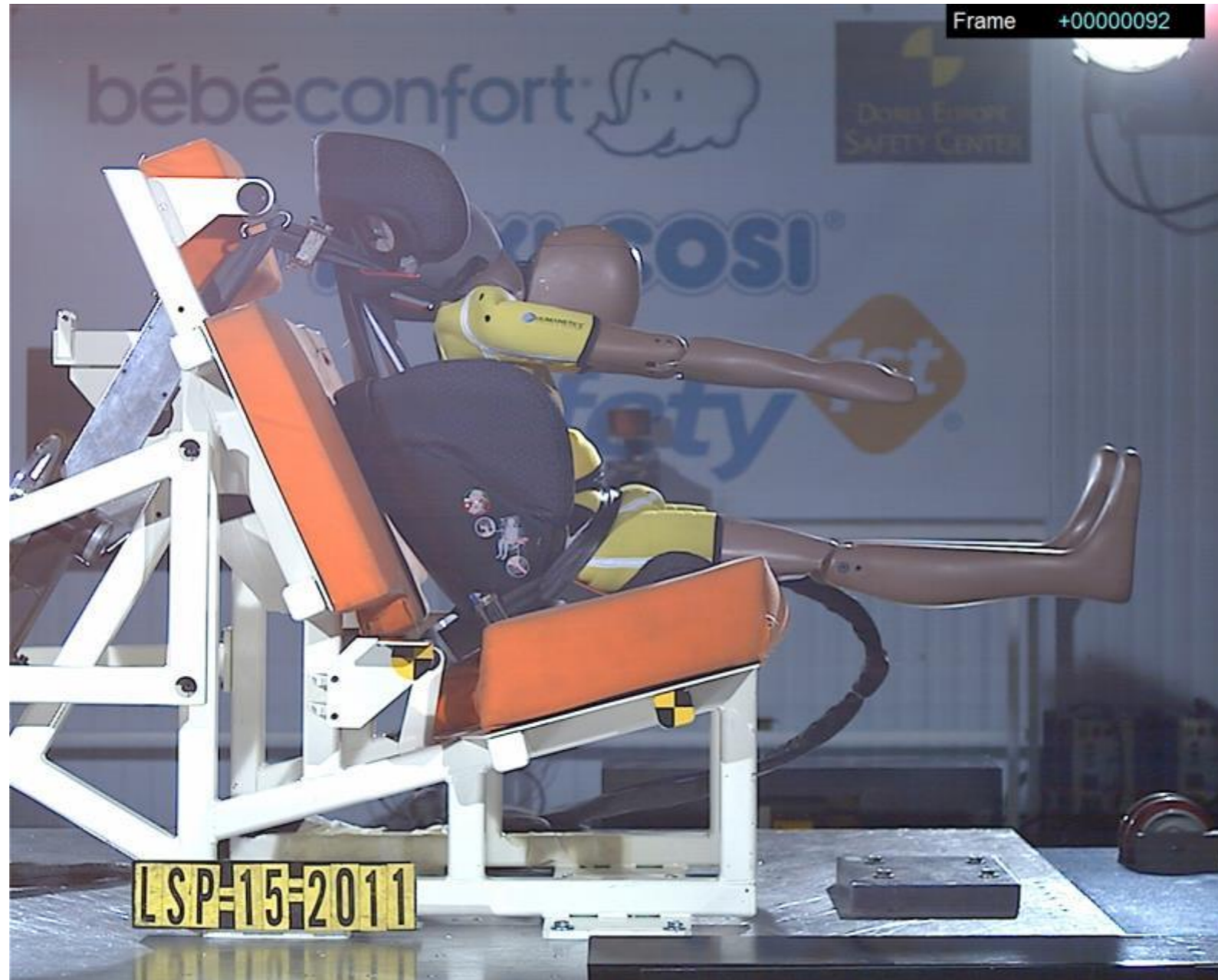
Normal Group 2 / 3 booster seat with dummy and silicone insert
