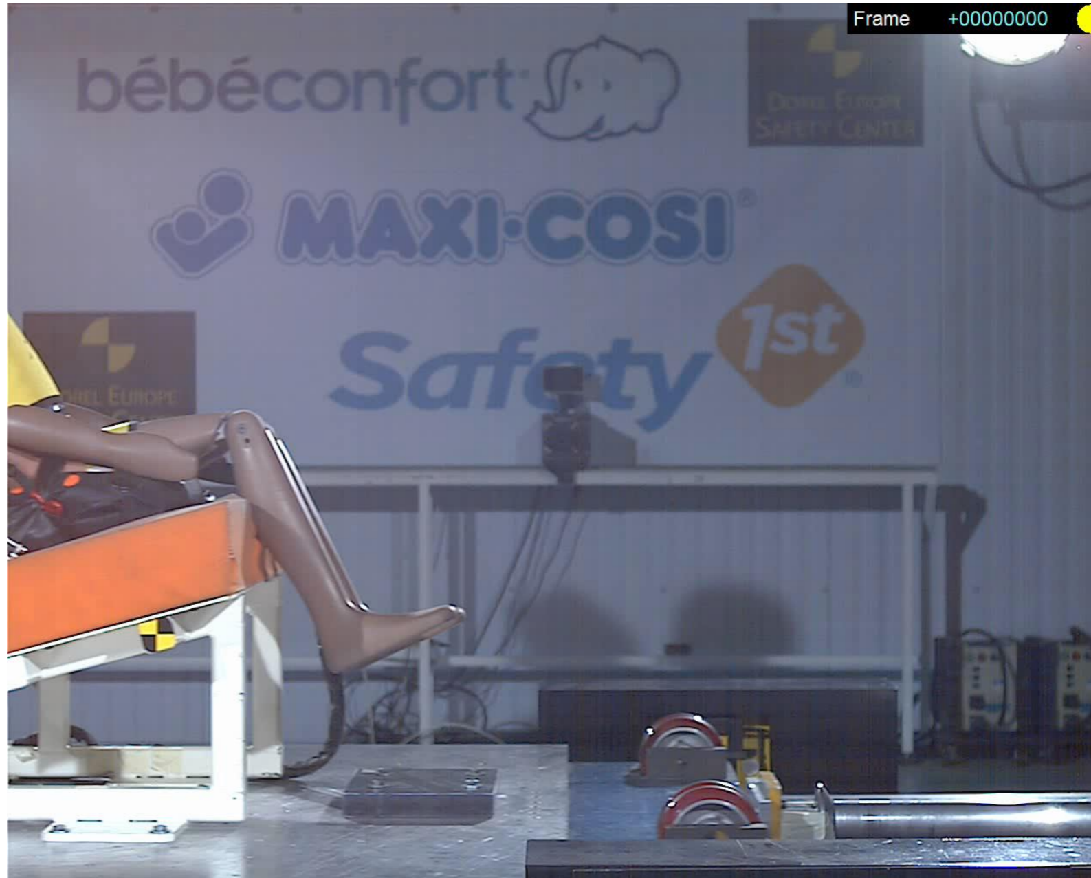
Inflatable Group 2 / 3 booster seat with normal dummy
