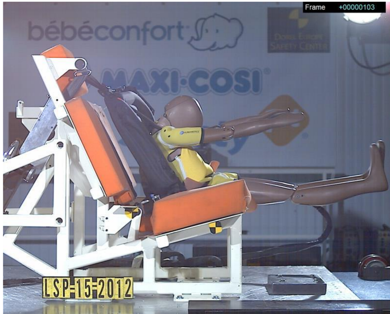
Inflatable Group 2 / 3 booster seat with normal dummy
