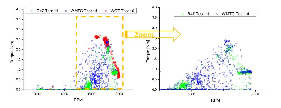
Larger area covered by WMTC  $\rightarrow$  maximized sampling in the part-load area Relatively little empty area between WOT Test and WMTC/R47 cycles
