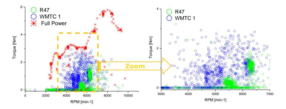
Larger area covered by WMTC  $\rightarrow$  maximized sampling in the part-load area
