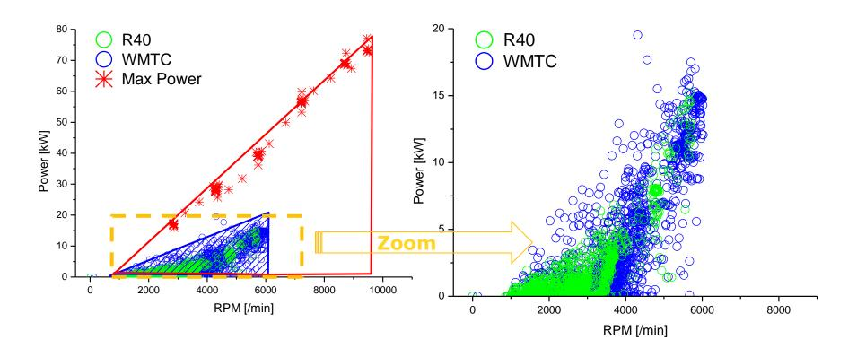
Larger area covered by WMTC  $\rightarrow$  maximized sampling in the part-load area
