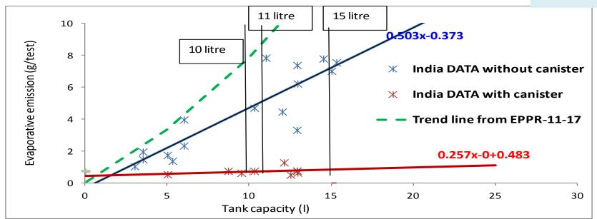
The increase in Evapo emission for increase in fuel tank capacity from 10 l to 11l (10% increase) and 10 l to 15l (50% increase) is shown below:
