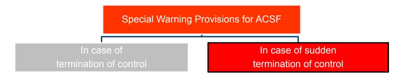
Any sudden termination of control caused by a failure of the system physical or functional failure shall produce immediately a distinctive driver warning by a [red] visual signal and either an acoustic signal that shall remain operational until the driver has resumed control.
