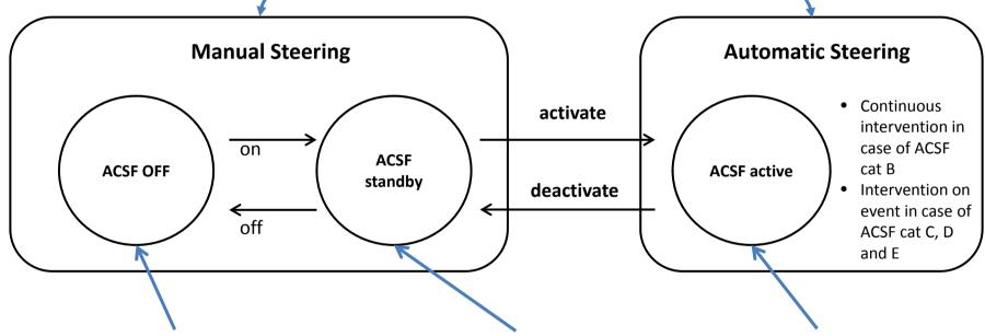
Manual mode does not have to be indicated to driver when system is OFF (except momentarily when the driver switches Off the system directly from Auto mode)
