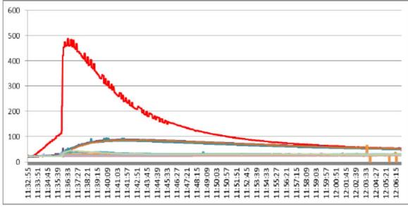
Thermal runaway of the cell happened 3 minutes later with the max. temp. of 487 °C.
