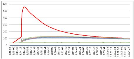
Thermal runaway of the cell happened 2 minutes later with the max. temp. of 565 °C.
