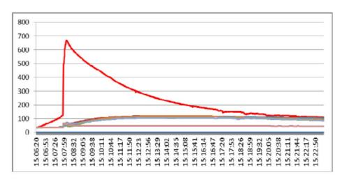
Thermal runaway of the cell happened 1.5 minutes later with the max. temp. of 668 °C.
