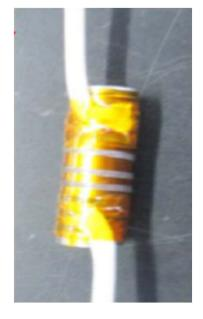
Heat the cell with resistive wire.
