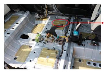
Position of thermal runaway cell
