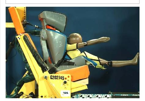
**Q6**Submarining on the test bench – 0.8 bar limit applied
