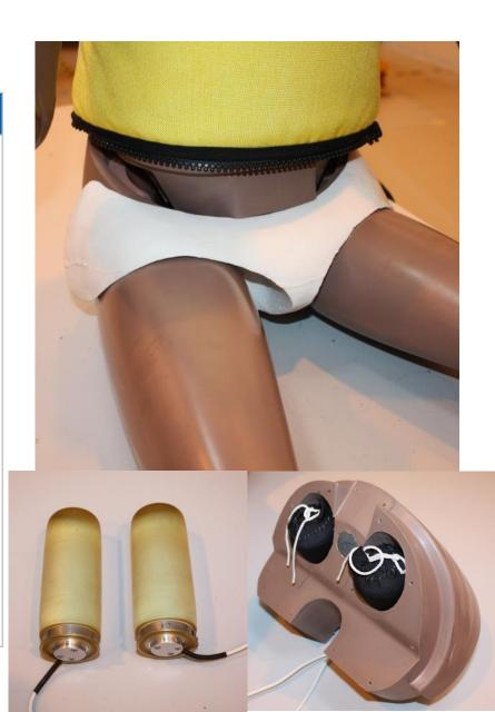
**Q10**Submarining on the test bench
