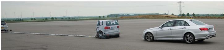
Test is passed: No collision and no steering around the obstacle
