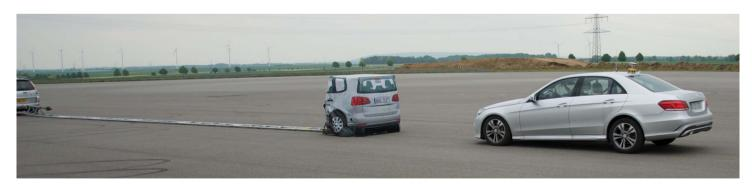
Test is passed: No collision and no steering around the obstacle
