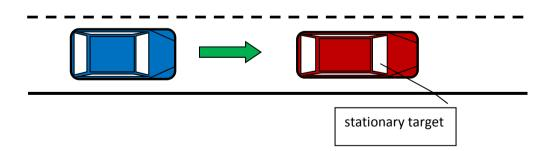
Test is passed: No collision and no steering around the obstacle
